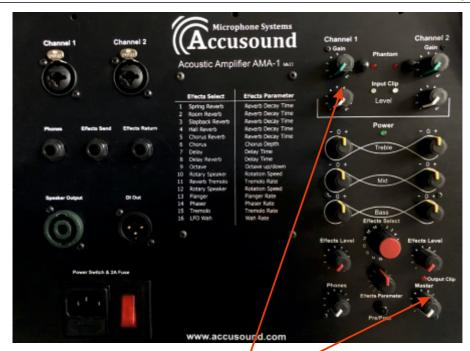
playing your harp until the LED starts to illuminate RED. Now turn the green knob slightly anti-clockwise so the LED only illuminates green, perhaps with a very occasional red flash. Don't be concerned if the LED does not flash Green, it simply means that your instrument has a low, but probably useable signal. Next turn the white "Master" knob, bottom right, to 4 or 5 and turn the white knob just under the green "Gain" knob to 3 or 4.
